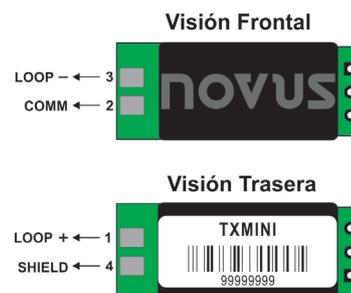
Fig. 3 – Salida 4-20 mA (sin M12)
