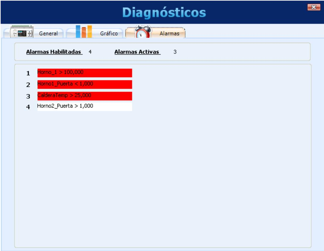
The screenshot shows the 'Diagnósticos' (Diagnostics) window with the 'Alarmas' (Alarms) tab selected. At the top, there are three tabs: 'General', 'Gráfico', and 'Alarmas'. Below the tabs, the status is shown as 'Alarmas Habilitadas 4' and 'Alarmas Activas 3'. A list of four alarms is displayed:
